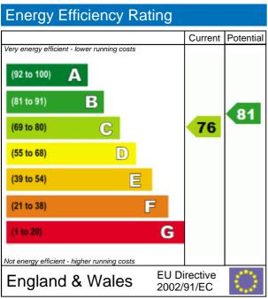
The energy efficiency rating is a measure of the overall efficiency of a home. The higher the rating, the more energy efficient the home is and the lower the fuel bills will be.
